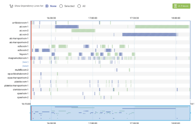
FIGURE 2. Yeast Cell Lysis, Sample Re-array and NGS Library Prep Automation Control Software (ACS) Protocol Runs; Two (2) Yeast Cell Lysis ACS protocol runs were executed in ~3 hrs, each processing two (2) 96-well microplates; two (2) Sample Re-array ACS protocol runs were executed in ~45 min, each processing one (1) 384-well microplate; two (2) NGS Library Prep ACS protocol runs were executed in ~2 hrs, each processing one (1) 384-well microplate
